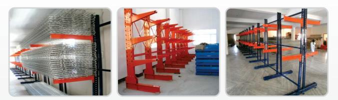
Ideal for storage of long items | Clear obstruction free storage bay | Easy height adjustments Can be customised for any need | Available for light duty and heavyduty applications
