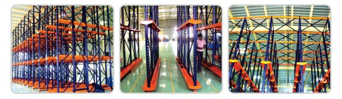
High storage ratio | Tall unit design | Reduced space for stacker movement | Maximum space utilisation Cost effective | Ideal for finished goods storage
